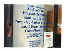
There are a varied group of small sign problems that need fixing, such as the Fire Hose sign that needs replacing. The required "Shipping & Receiving" tactile sign at the side of the door would be difficult to locate, but a small one could be placed on the pillar to the left. The Mail Room sign needs to be redone without the italics.
