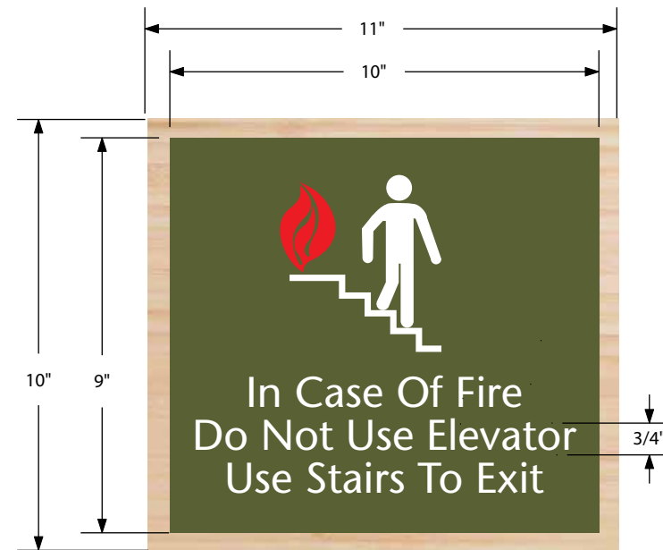
B Sign For Exterior Elevators Scale 1:4
