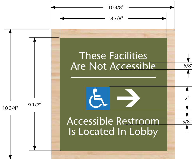
A Accessible Restroom Directional Sign Scale 1:4
