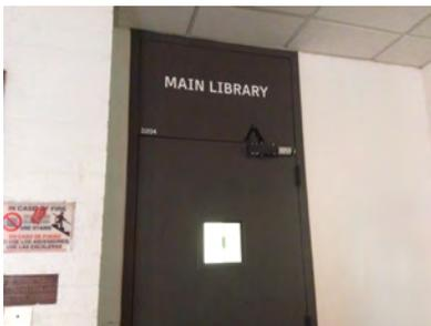
The last photo shows what is the major means of door identification throughout the facility, a tiny visual sign way far above the finish floor, and no accompanying tactile sign.
